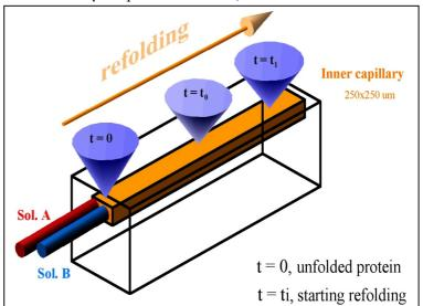
**Fig. 2** After rapid mixing, the refolding protein flows down a narrow capillary. Thus, the distance along the capillary represents the time after mixing as a function of flow speed.
