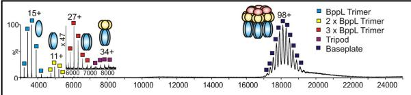
**Figure 1:** ESI-MS spectrum of the intact TP901-1 lactococcal phage baseplate (mass 1.769 MDa; m/z ca 18,000) and associated sub-complexes. Key: pink = distal tail protein (Dit); yellow = baseplate protein upper (BppU); blue = baseplate protein lower (BppL).
