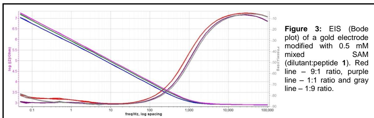
**Figure 3:** EIS (Bode plot) of a gold electrode modified with 0.5 mM mixed SAM (dilutant:peptide 1). Red line – 9:1 ratio, purple line – 1:1 ratio and gray line – 1:9 ratio.
