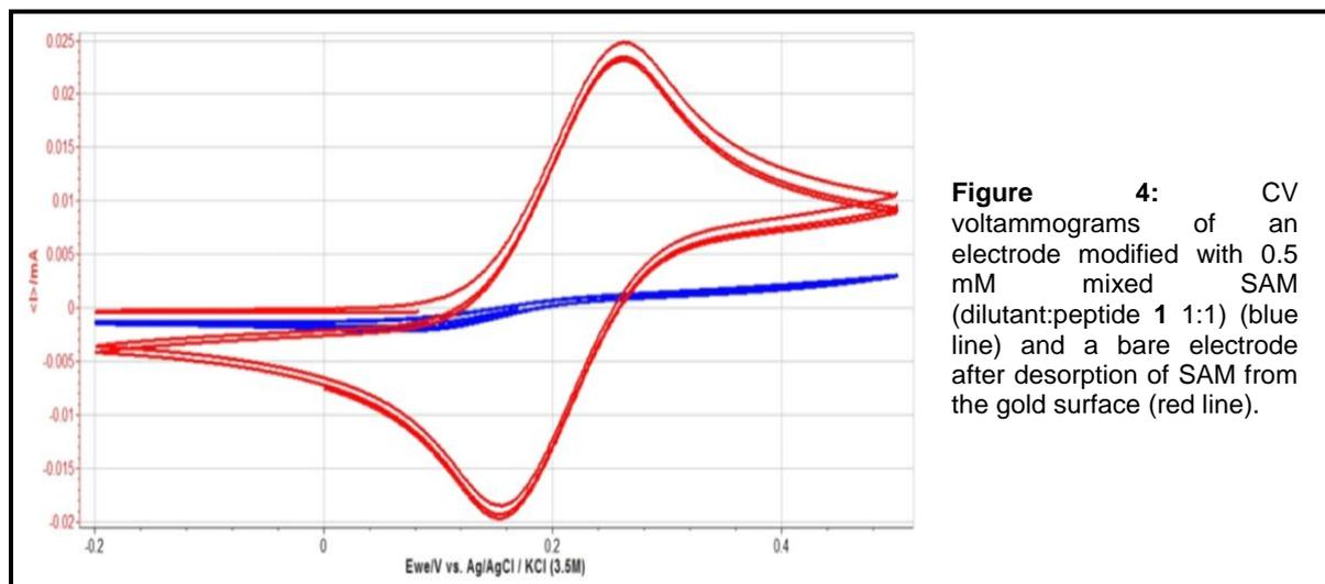
**Figure 4:** CV voltammograms of an electrode modified with 0.5 mM mixed SAM (dilutant:peptide 1 1:1) (blue line) and a bare electrode after desorption of SAM from the gold surface (red line).
