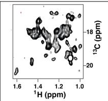
**Figure 3:** Two dimensional Ala $\beta$  HMQC spectrum of 1  $\mu$ M BIP NBD, measured at  $^1$ H frequencies of 950 MHz.
