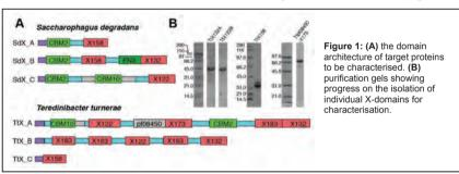
We are currently working on expressing and purifying these domains (Figure 1B) with the aim of combining structural studies together with biochemical, spectroscopic and redox analyses to gain a thorough understanding of X-domain function. We will then seek to exploit the knowledge gained through enzyme engineering to ensure maximal enzyme turnover during biomass degradation whilst also investigating other potential applications for these domains.
